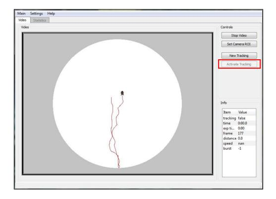
Whenever a fly jumps off the platform there will be a sound. For a 15 minutes experiment it suffices to put the fly carefully back on the platform (brush) and press "Activate Tracking" again. For a 5 minutes experiment it is necessary to start the recording all over again, therefore put the fly back on the platform and choose "New Tracking"; keep all of your settings, overwrite the existing file and choose "Activate Tracking" again.
